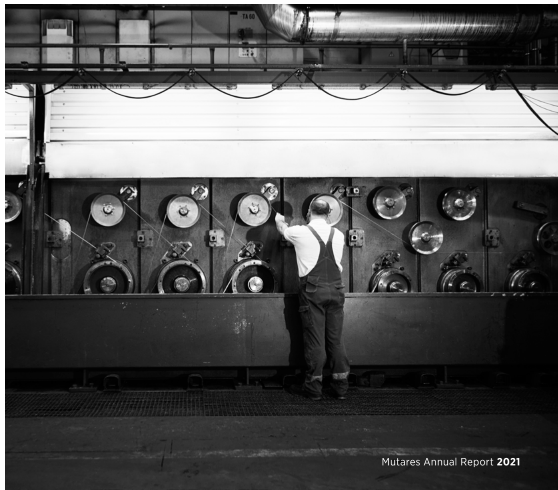
Employee checking machine, which is making copper wire thinner by extending it
