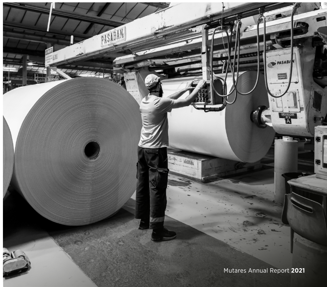
Cutting machine bringing the cardboard in the right format
